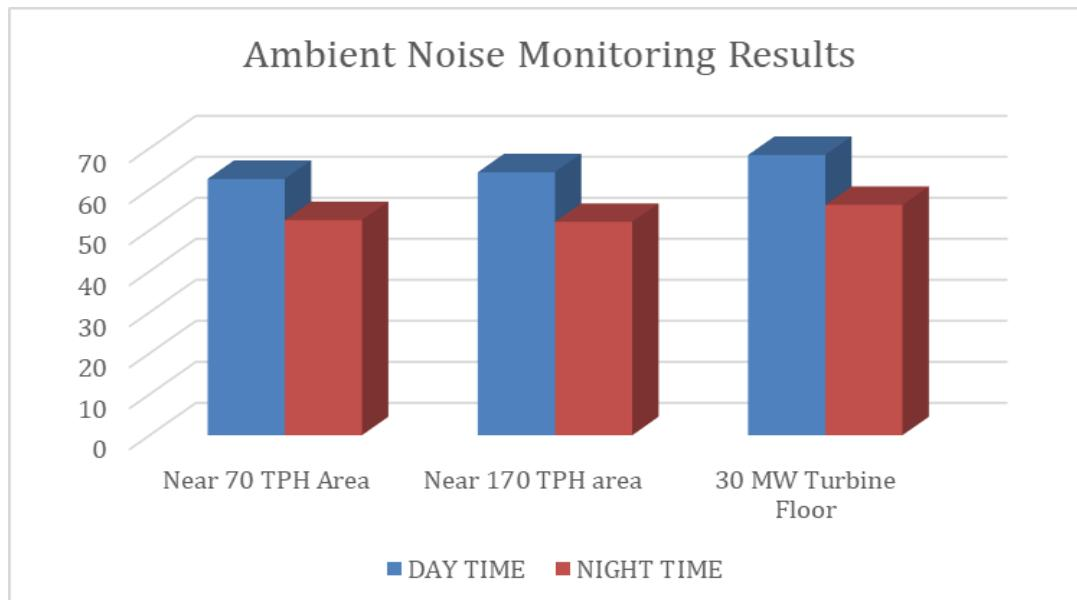
**Figure-3.5: Day and Night Time noise Level at all Monitoring Locations**
